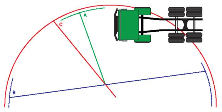
Tests have shown that the true location of the turning center is further to the rear than midway between drive axle sets (where applicable)
